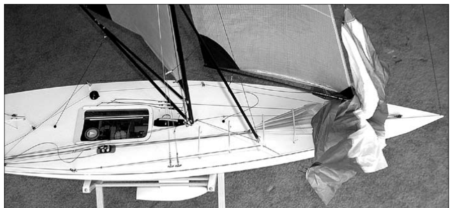
As the boat is turned on to a run, the spinnaker winch is actuated. The trolley moves forward pulling up the halyard. At this point, when the elastic is running through the trolley free of stopper knot contact, tension is minimal on the foreguy, topping lift, sheet and afterguy.
