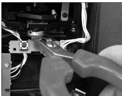
Figure 7. Clipping the potentiometer's leads. This is the point of no return. Do this and you void your warranty.
