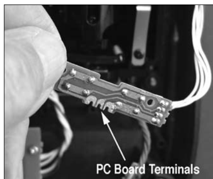
Figure 9. This is what the PC board should look like before you reinstall it in the case. Make certain that the gaps between the pads have not been violated by solder.
