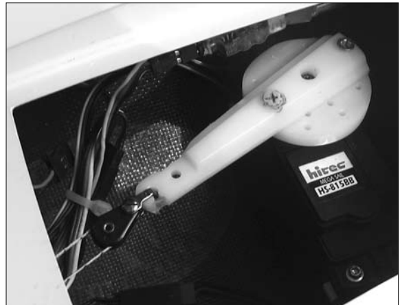
Figure 1. Single pulley block on sail servo arm. All photos by Bill Mullica.
