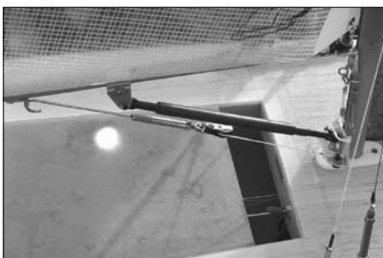
Below: This vang uses a spring to hold the boom up and an eccentric system to change the angle of the boom, depending on its distance from the centerline. Very Hi-Tech.
