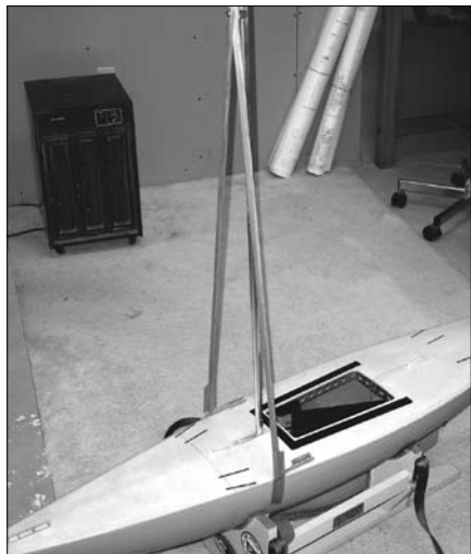
Used to stand the mast vertical to the hull
