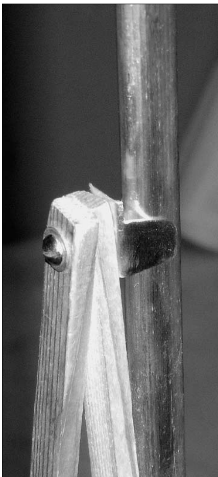
The top snaps to the mast. If both legs are equal length, then the mast will stand vertical (Remember your geometry 101? And you thought you'd never have a use for it?)
