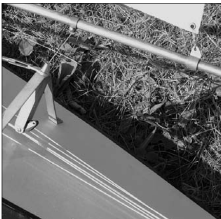
Often blocks are used in conjunction with the fairlead, to decrease friction.
