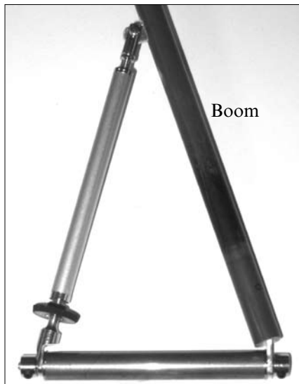
This photo shows the basic assembled gooseneck, ready to be glued to a mast or deck post (if using an offset gooseneck). Basic Tangs can be used as simple attach points for the boom and vang, although a Sails Etc. compression strut is used here.
