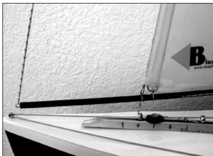
Figure 3. Adjustable jib swivel position.
