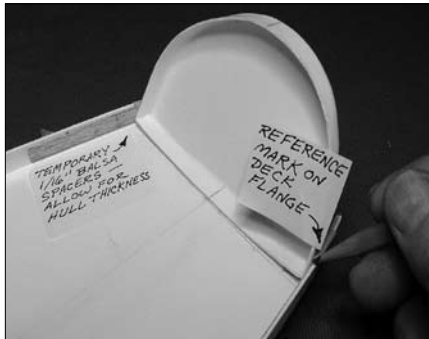
Transferring the transom location to the outside of the deck flange. Editor: The illegible note on the left reads: Temporary 1/16 inch Balsa spacers allow for hull thickness.
