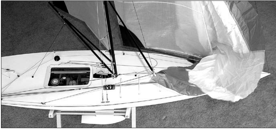
The trolley is going forward and is in the area near the mast. The halyard has the spinnaker about half way up. The elastic passing through the trolley has made contact with the foreguy's stopper knot and is now pulling on the topping lift, sheet and afterguy.
