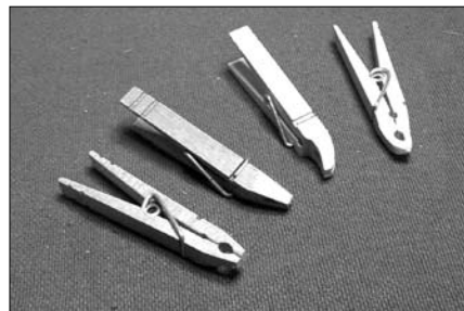
Customized clothes pins make great modeling clamps. Pins on the left have angled jaws. Pins on the right have curved jaws. They were shaped on a disc sander in just a few seconds each.
