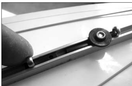
Figure 5. Free sliding eyebolt with spacer.
