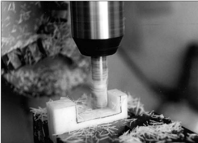
Photo #2 To reduce the set up time, I mill three pieces at once. This is the outside part that connects the vang and boom.
