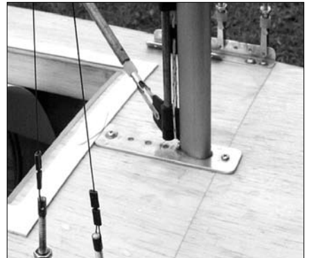
The simplest mastcrane is a flat piece of material, rigid enough to withstand the forces it encounters.
