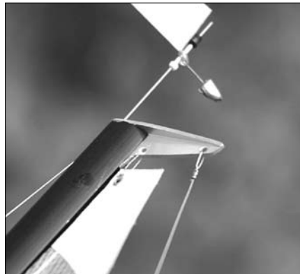
Another inventive modeler is using an extruded shape then modifying it to a streamlined shape. Very light, very strong.
