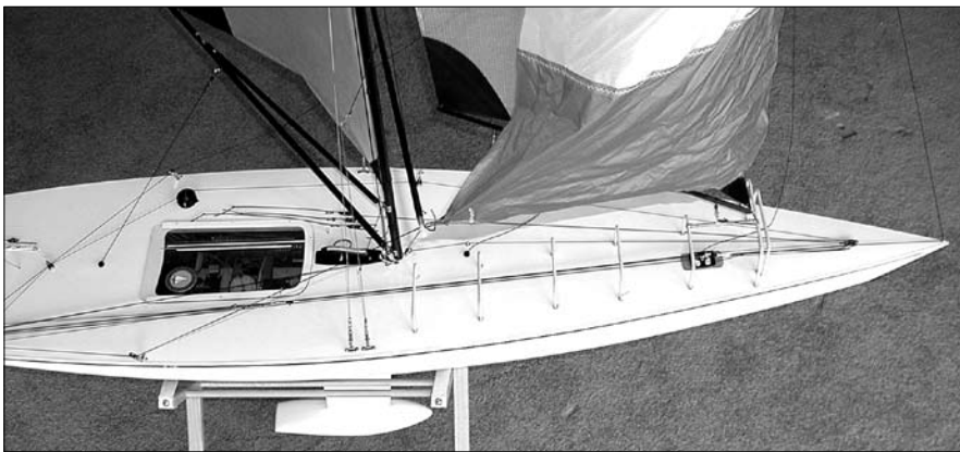
The trolley is at the end of its run. The halyard has brought the spinnaker head up against the block where the jibstay meets the mast. The retractor line is slackened. The trolley is all the way forward and providing the needed tension on the topping lift, sheet and afterguy.
