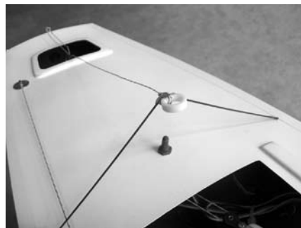
Figure 6. Waterproof switch and mainsheet bridle.
