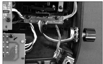
Figure 11. This is what the new auxiliary pot one installation should look like when you're done. It's really pretty simple.
