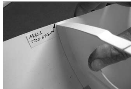
This forward bulkhead is pressed into the hull with the centerlines aligned. The hull edge is above the bulkhead and must be trimmed or sanded to fit.
