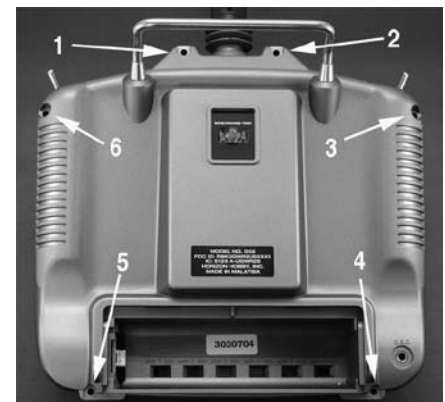
Figure 4. Locations of the six screws that hold the transmitter back in place.
