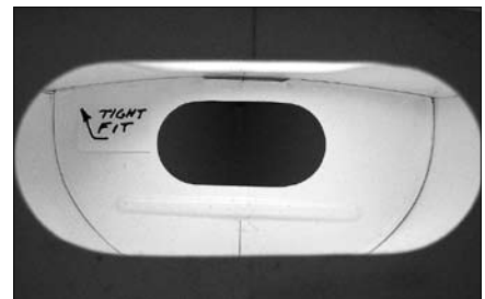
This hull is trimmed and the bulkhead joint is tight.
