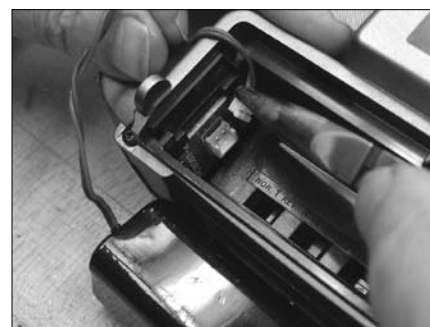
Figure 3. Removing the transmitter battery pack. Try pulling it out without the pliers first.
