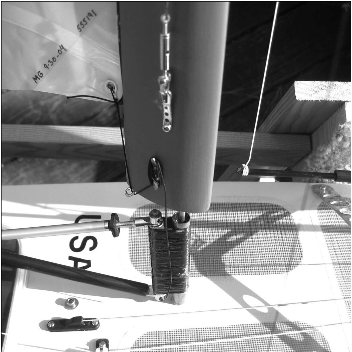
Close up of mast step and offset gooseneck.
