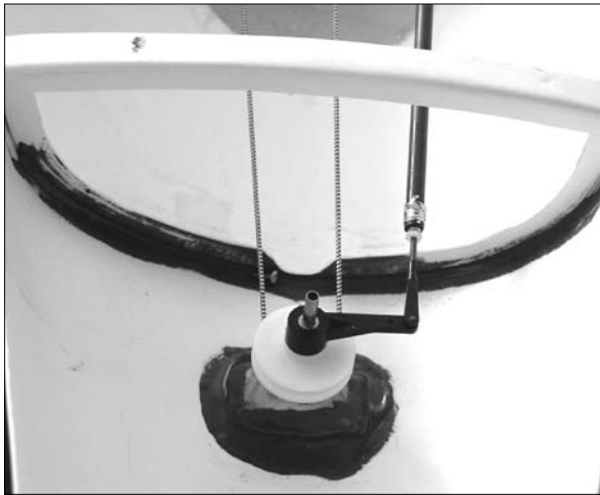
Photo F. The Rudder Tube Sheave is made from a nylon screen door wheel. The wheel is drilled and shimmed to fit the rudder post.
