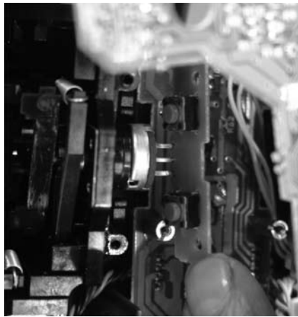
Figure 14. This is auxiliary pot two... ready for clipping. Don't worry, you've already voided your warranty.
