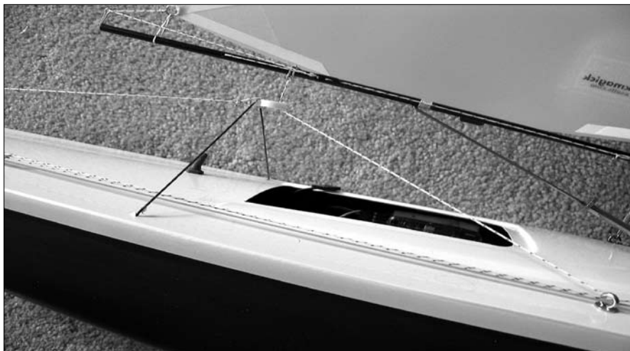
Figure 7. Adjustable mainsheet position.
