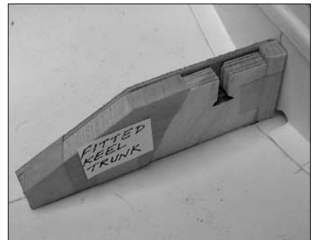
Here, the keel trunk parts are fitted for better support, fore and aft.
