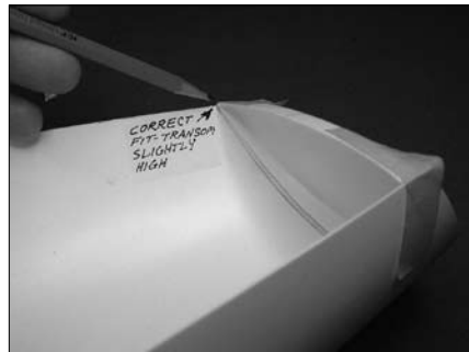
Here the hull is trimmed to match the transom. Transom is held temporarily with tape. A line is scribed along the transom flange to use for alignment. A hull reference mark is on the right side where the deck flange markings were transferred.
