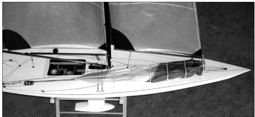
When retracted the spinnaker is neatly furlled close to the deck by the hoops. The trolley is well aft and is keeping elastic-loaded tension on the foreguy that keeps the pole snug against the forward side of the mast.
